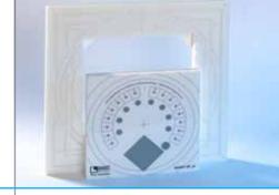
The *QUART SP\_dI* phantom is designed to be used for QA/QC routine testing in Digital and Conventional X-Ray applications ranging from DR, CR to Fluoroscopy equipment.
