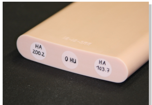
QRM-Bone in the Bone Calibration Phantom
